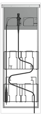
To avoid damage to distal ends, the rack is made of 2 separate and mobile parts enabling a perfect adjustment according to the size of the endoscopes.
