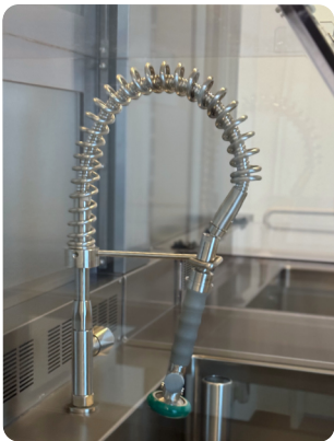
Cleaning spray head for cold water or deionised water mounted beneath the protective hood
